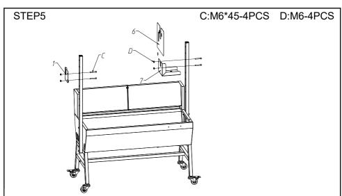
The fire shield plate is positioned onto the motor support plate, which is then aligned with the support pipe hole, adjusted to the appropriate height, and secured in place using M6\*45 hexagonal screws and M6 flange nuts. The Spit bracket is then placed at the corresponding position on the other support pipe.
