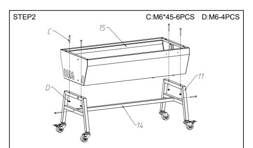
Fix the support foot and Grill body with M6\*45hexagon screws and M6 flange nuts .
