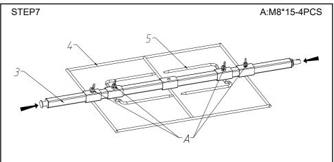
As shown in the picture above, secure the food on a grilling fork or Fixed mount, and then secure the grilling fork or Fixed mount to the grilling rod using an M8\*15 butterfly screw.
