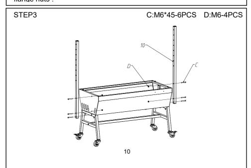
Fix the bracket and furnace body with M6\*45 hex bolts and M6 butterfly nuts.
