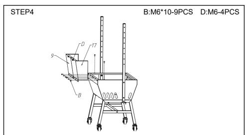
The left and right windshields and grill body are fixed with M6\*10 hexagon screws, and the left and right windshields are fixed with M6\*10 hexagon screws and M6 flange nuts.
