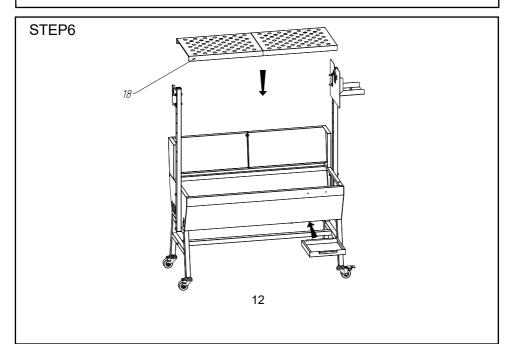
Place the charcoal tray in the grill body .Insert the slag tray under the grill body
