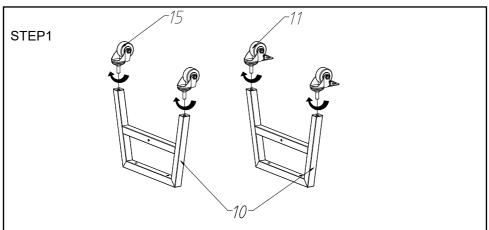
Install four casters on the support foot, rotate and tighten them in the direction of the arrow, and install casters 1 (with brake) on the same support foot.
