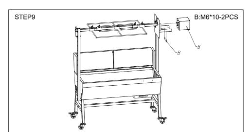
Place the motor on the motor support plate and insert it into the Spit, and then lock it with M6\*10 hex socket screws. The installation is complete. Put the charcoal on the charcoal plate, light the fire, you can roast sheep and other large foods
